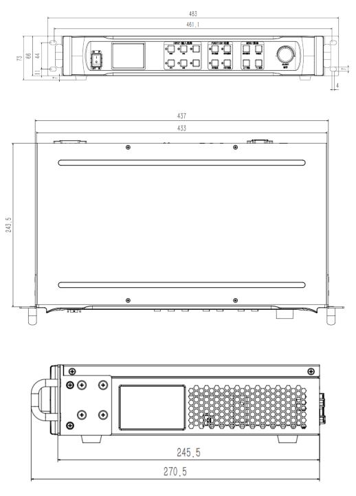
Unit: mm Unmarked linear and angular dimension tolerances comply with GB/T1804-M
